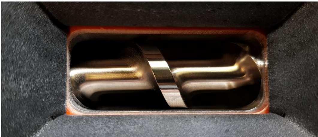
image 18 empty hopper with visible screw
